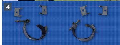
Figure 3: Accumulator mounted with non-approved wide clamps (from Service Bulletin 724-29-1018)
