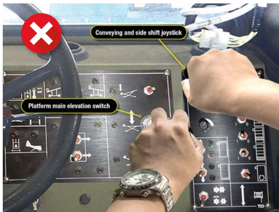
Incorrect switch selection for cargo deck adjustment
