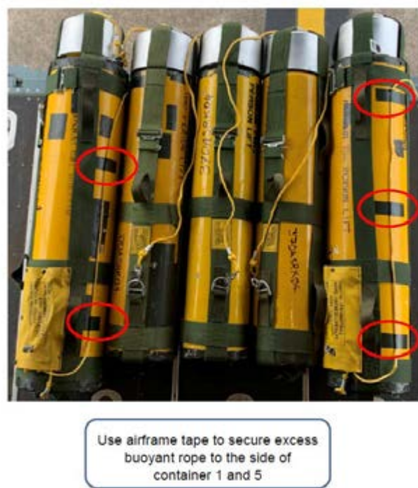
Figure 2. Amended ASRK rigging procedure
