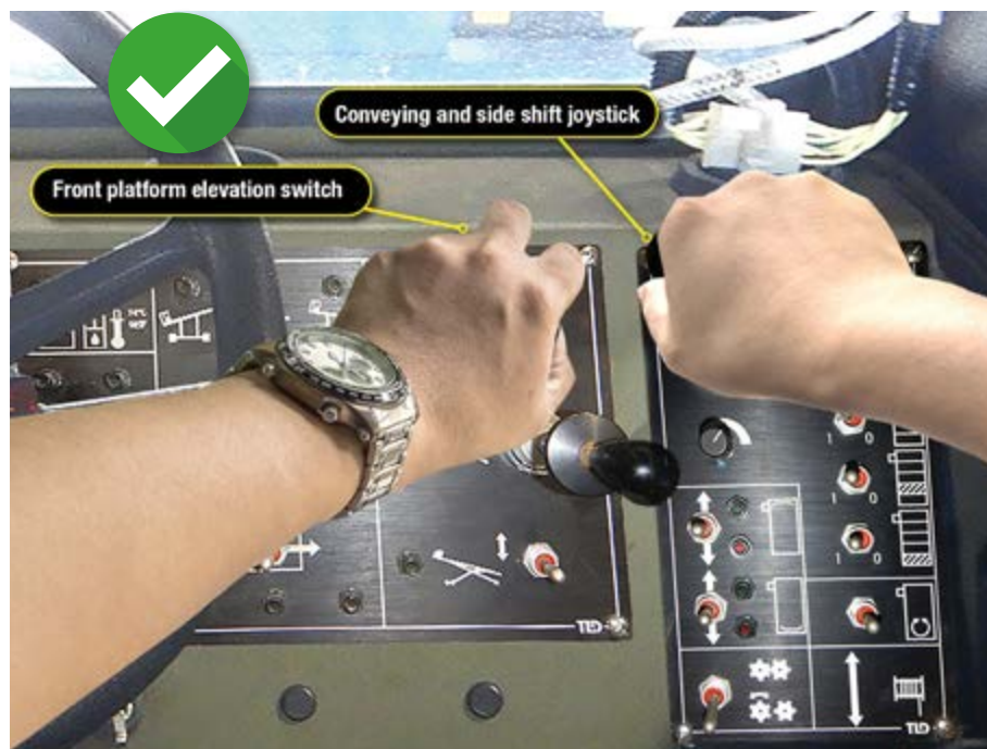
Correct switch selection for cargo deck adjustment
