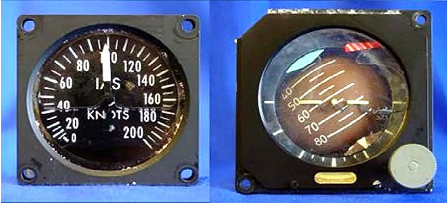
Standby instruments show 100 kts/65 degrees nose down and 30 degrees right wing low.
