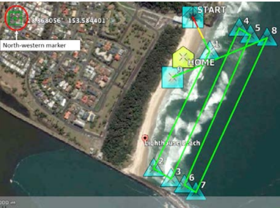
Figure 4: Image uploaded onto GCS with planned mission overlaid. Source: Remotely piloted aircraft system operator, annotated by ATSB.
