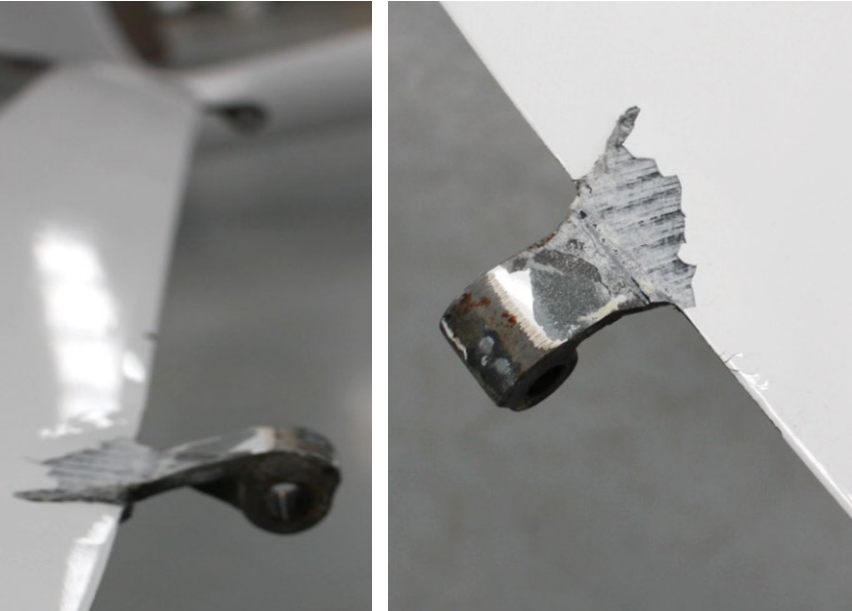
Hinge over-extension and supporting structure damage
