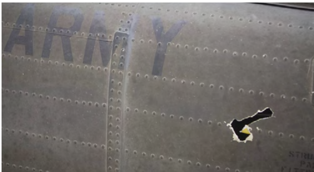
Figure 5–2. Shrapnel damage during combat may need to be repaired without the usual tools or resources
