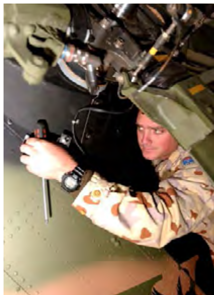
Figure 15–3. Working in confined spaces requires dexterity and flexibility as, among other things, tools are difficult to use
