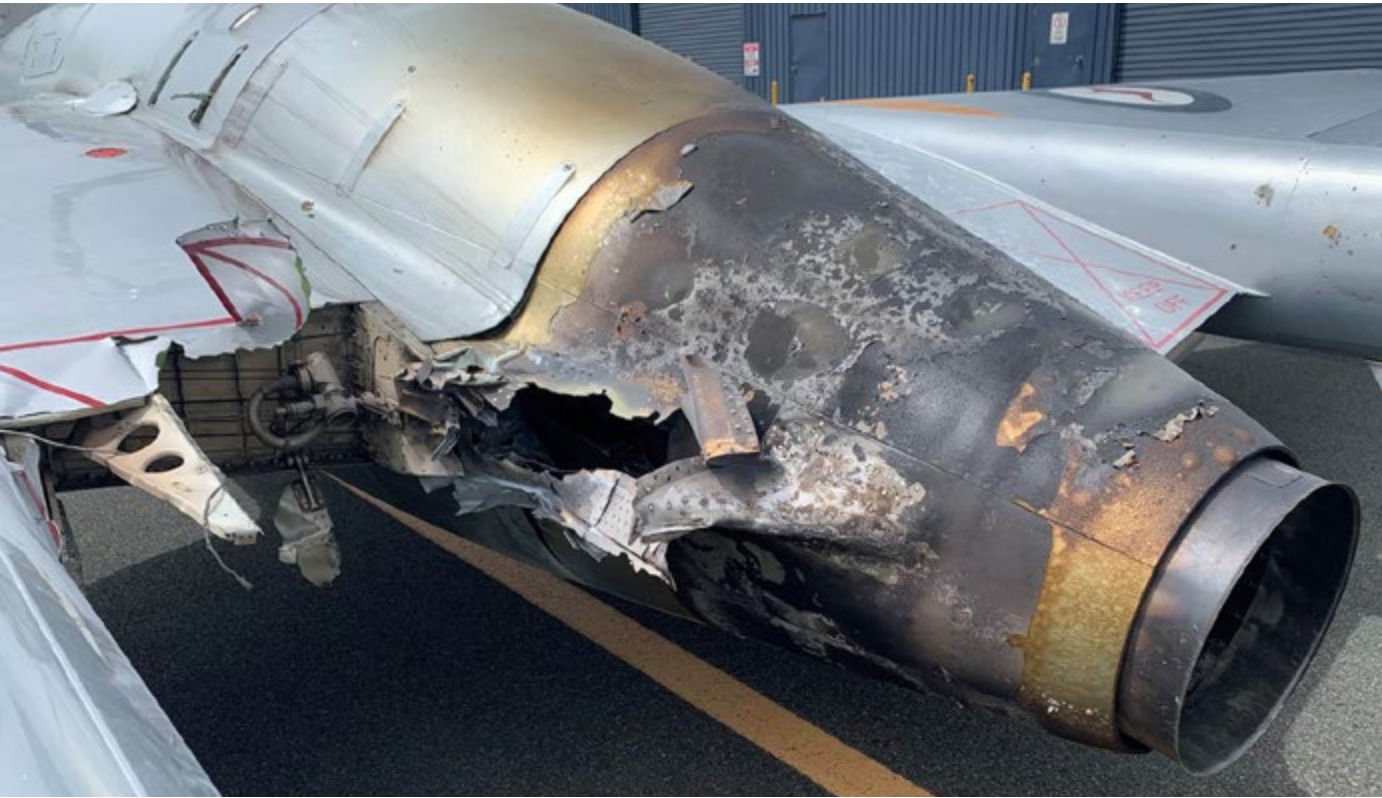
Gaping hole adjacent to fire extinguisher with deformation of material directed from the engine
