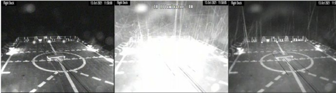
CCTV screenshot before, during and after activation of IR illuminator pre-accident
