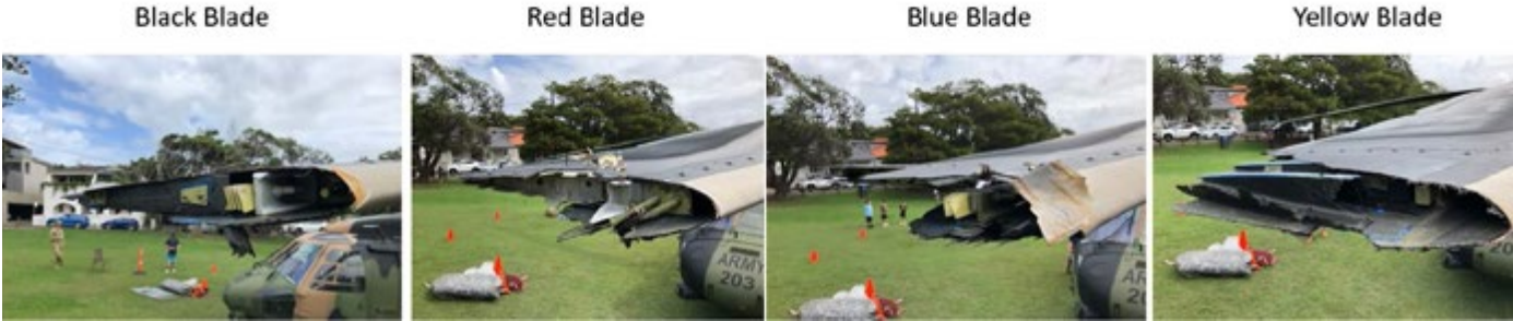
Blade tip damage
