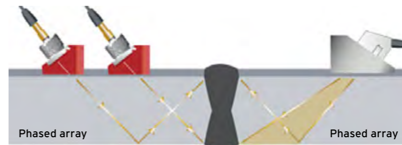
Figure 2: Comparison of conventional UT and phased array UT principles Source: 'Phased Array – an overview', ScienceDirect Topics
