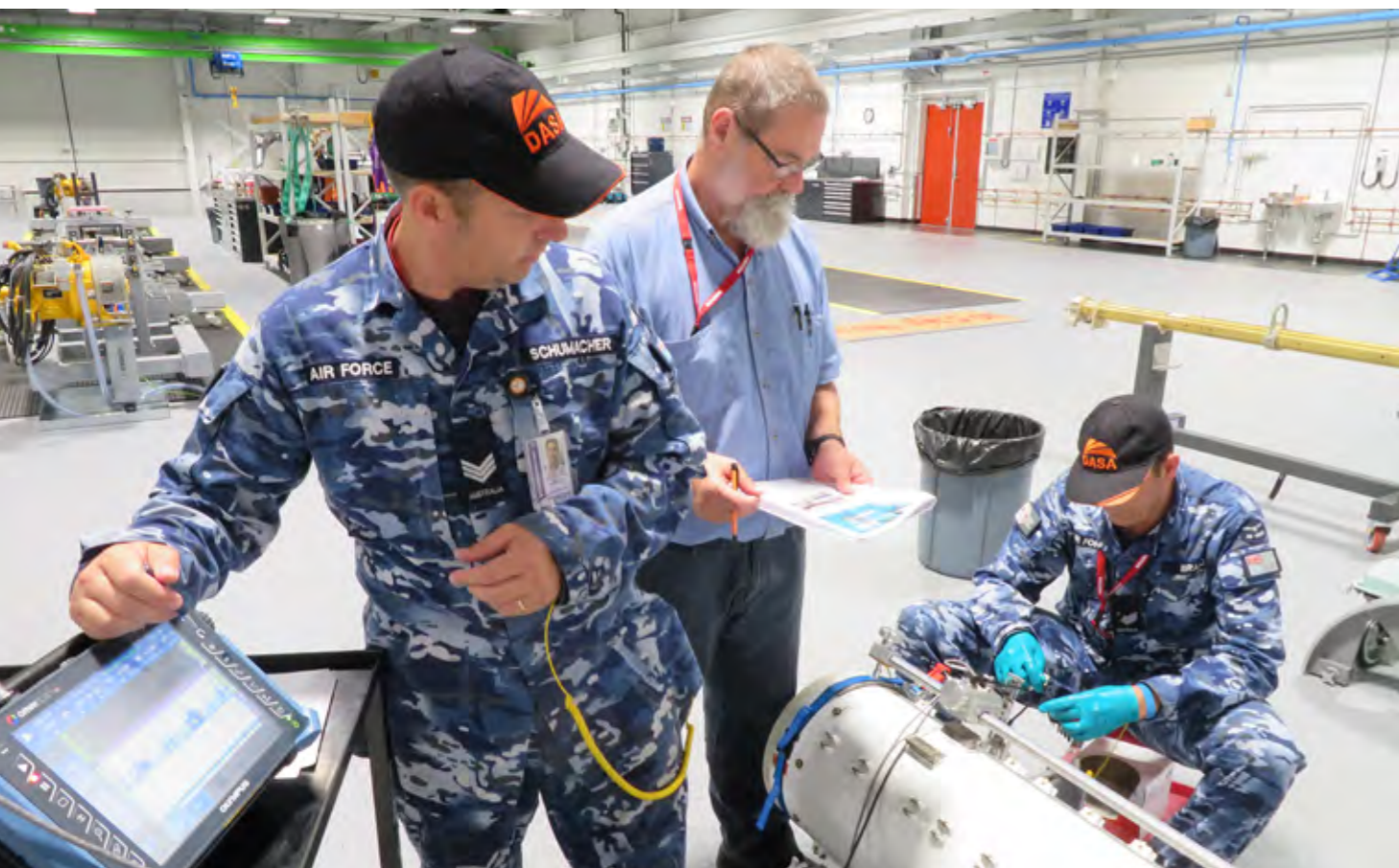
Figure 4: Staff from NTD Engineering conducting Missile Airframe PAUT Test Procedure
